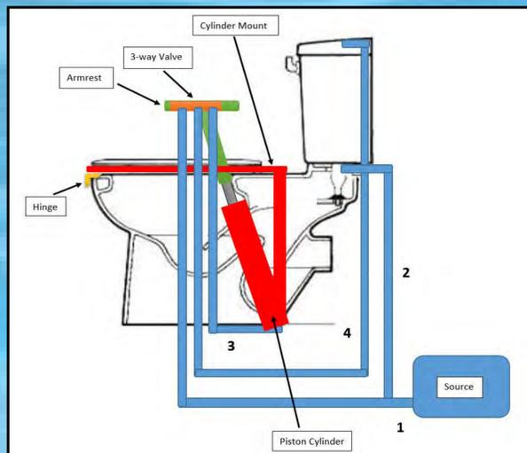
**Lifting:** The valve handle is turned to the 'lifting' position, which connects the water source to the hydraulic cylinders. This allows for flow into the cylinders, thus pushing the pistons and raising the seat.
