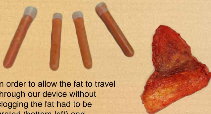
In order to allow the fat to travel through our device without clogging the fat had to be grated (bottom left) and pretreated through a series of needles (top left) to reduce the tissue size (bottom right).
