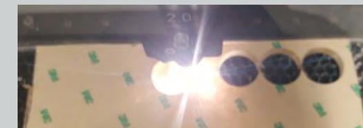
Laser cutting disks out of acrylic prepped with adhesive
