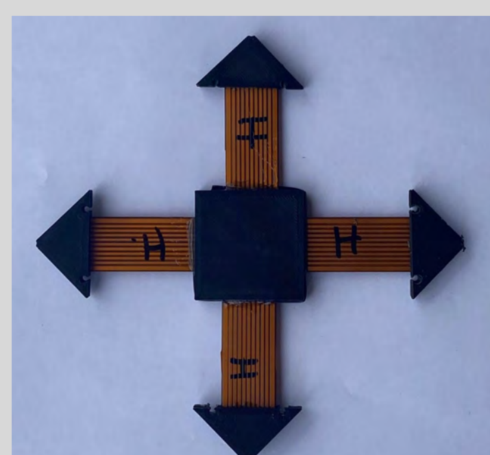
Figure 3. Fabricated prototype made with PLA, Copper, and Kapton tape.
